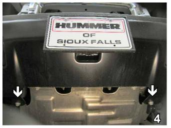
Just below the bumper, remove two metric bolts with the 18MM socket. Pull the metal bumper forward and disconnect the fog lights. Set bolts and metal bumper aside to be reinstalled later.
