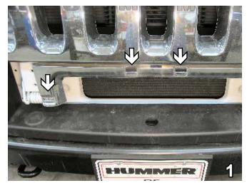
Pull the center grille insert forward to release the four clips, one on each side and two in the middle. Set insert aside to be reinstalled later. The passenger's side is shown in the photo above.
