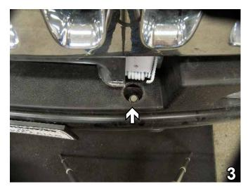
3. Using the 18MM socket, remove one metric bolt from the top of the bumper. Do this to both sides of the vehicle. Set bolts aside to be reinstalled later.
