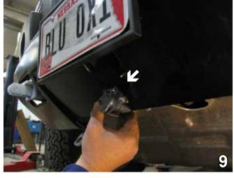
Using the 1" self tapping screw, install the electrical bracket just below the license plate bracket while ensuring enough clearance for the bracket cover to open.
