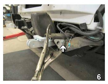
6. Insert the baseplate weldment into the tow hook opening and align the backing plate with the outside tow hook hole, 1/4" forward of the frame rail, clamp in place and install the 4 1/2" hex bolt, 1/2" lock washer and 1/2-13 hex nut. Do this to both sides of the vehicle.
