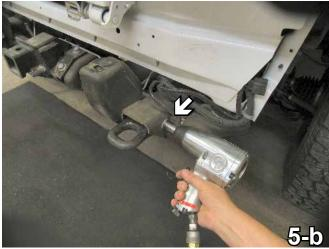
5. Using the 18MM socket, remove three metric bolts from the tow hook, two on the inside (see photo 5-a) and one on the outside (see photo 5-b). Pull tow hook forward and set aside. Do this to both sides of the vehicle. The tow hooks will not be reinstalled. Please return them to the customer.
