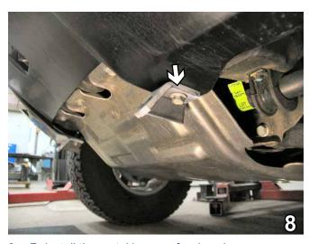
Reinstall the metal bumper fascia using upper existing bolts but do not tighten completely. Install the convenience link weldment to the lower existing bolt, tighten all bolts completely and reinstall the rubber inserts, fog lights and grill insert.
