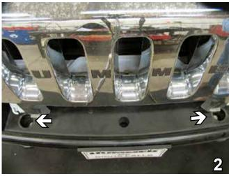
2. Remove the two rubber inserts from the top of the bumper. Set the rubber inserts aside to be reinstalled later.
