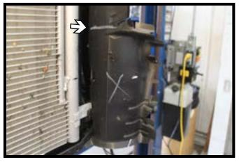
Trim the plastic shielding just below the notch as shown. Do this on both sides of the vehicle.
