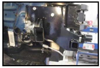
14. Prior to drilling and installing the remainder of the baseplate bolts, flatten the three (3) tabs of the horn bracket so it will sit flat on the face of the side plate. Also it may be necessary to ream out the slot to accommodate the hardware (left).
