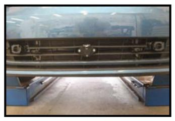
18. Hold the fascia as close to its original position, mark and trim the fascia around the convenience links and attachment tabs. Reinstall the fascia and grille.
