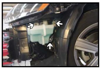
Using a 10MM socket, remove the three
