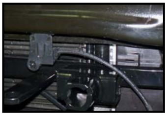
16. Reinstall the air temperature sensor.
