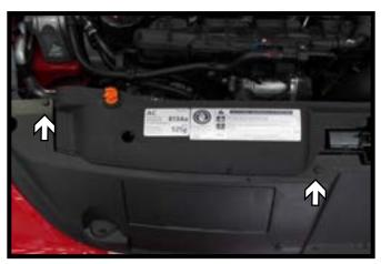
1. Remove the four (4) push pins from the top edge of the radiator cover. There are two (2) on each side. Then remove cover from vehicle.
