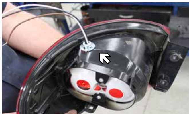
Possible location of the BX8869 Bulb & Socket Wiring Kit
