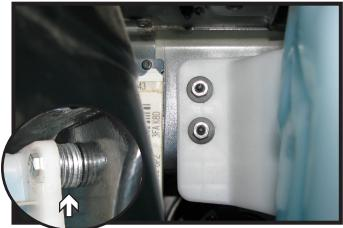
20. Put the washer reservoir in place on the back two studs and loosely reinstall the two (2) hex nuts. Use the 6MM hex bolt provided on the front hole with flat washers as spacers to prevent webbing from rubbing a hole in the reservoir tank. Tighten the back nuts and reconnect all the electrical and fluid lines to the reservoir.
