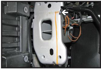
12. Using a reciprocating saw, cut the webbing horizontally flush with the top of the frame rail then vertically flush with the side of the fram rail all the way down. Do this on both sides of the vehicle.
