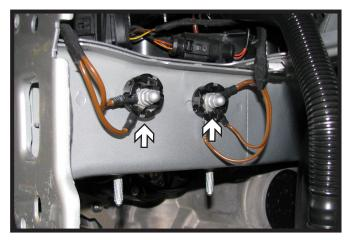
10. **2011 Model:** On the driver side, using a 10MM socket remove the two (2) nuts holding the ground wires. Move the ground wires out of the way. Cut the studs flush with the frame rail.
