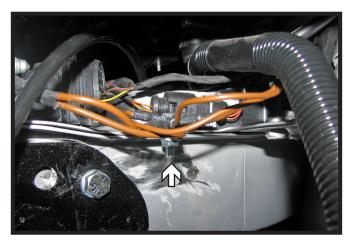
21. On the driver side, drill a 1/4" hole in the edge of the frame. Attach all the ground wires together with a 1/4"-20 x 1" bolt and 1/4"-20 lock nut.
