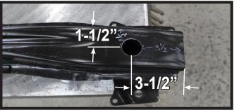
16. On the passenger side, enlarge the hole on the front of the metal bumper just forward of the center of the frame end. Use a reciprocating saw and enlarge the hole or drill out with an 1-1-4" hole saw.
