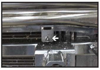
18. Drill a 1/2" hole in the plate as shown above and insert temperature sensor into hole.
