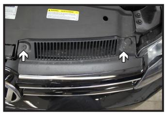
1. Using a T25 Torx, remove the two (2) screws from the top edge of the fascia. There are two (2) on each side.
