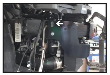
17. Slide the baseplate into position, centering the slot in the baseplate horizontally with the existing hole in the frame. Flush the baseplate with top of the frame. Level and clamp the baseplate into position.
