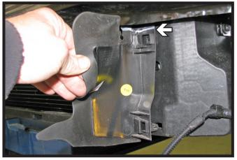
14. Trim the plastic shrouding off just below the bumper. Do this on both sides of the vehicle.
