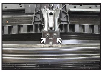
9. Using a T30 Torx, remove the two (2) screws from the middle of the bumper and set the bumper aside.
