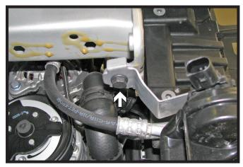
11. Using the 13MM socket, remove the bolt from the horn bracket. Unplug the electrical connection and set the horn assembly aside. Do this on both sides of the vehicle.
