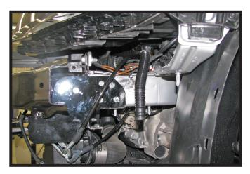
23. Attach the permanent baseplate safety cables to the provided convenience link on the baseplate. The photo above shows the recommended installation of the cables to frame of vehicle. Additional options may interfere with suggested mounting; in this case, secure the cables to a solid piece of the frame as described in the General Information sheet. Be sure the safety cables do not rub against any hoses or moving parts. Do this on BOTH sides of the vehicle.
