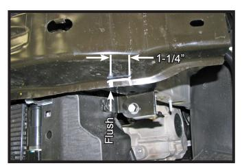
15. **2011-12 Models:** Mark the lower lip of the bumper flush with the outside of the frame rail and 1-1/4" wide. Remove the section of the bumper lip for baseplate clearance.
