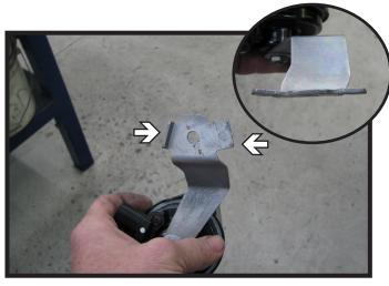
Flatten the horn bracket tabs on the passenger side only. Reattach both horn brackets and plug in the electrical connections.
