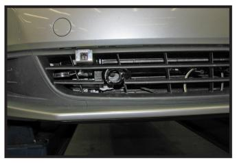
24. Reinstall the stryofoam bumper. Hold the fascia as close to its original postion, mark and trim the fascia around the convienence links and attachment tabs. Reinstall the fascia.
