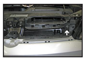
3. Using the T30 Torx, remove the two (2) bolts from the lower grille, one (1) on each side.
