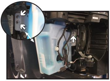
10. On the passenger side, using a 10MM socket, remove the three (3) nuts from the washer reservoir. There are two (2) on backside and one (1) in front. Disconnect all lines and set the washer reservoir aside.
