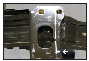
13. Temporarily reinstall the metal bumper. to its original position. Mark the back side of the webbing where the frame webbing was removed. Do this on both sides. Remove the bumper, then cut out the areas with a reciprocating saw. Then reinstall the bumper.
