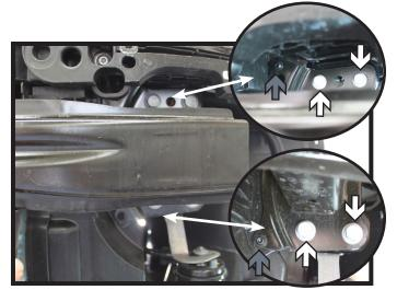
8. On the outer edge of the bumper, using a T30 Torx, remove the two (2) screws (gray). Then using a 16MM socket, remove the four (4) bolts (white). Do this on both sides of the vehicle.
