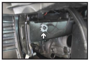
10. **2012-13 Models:** On the driver side using a 10MM socket remove the one (1) ground wire nut. Move the ground wire out of the way. Cut the stud flush with the frame rail.
