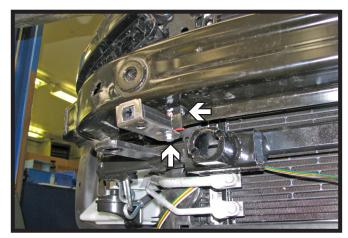
22. **Optional:** Drill a 1/4" hole in the center of the metal bumper. Attach the breakaway bracket to the bumper with 1/4"-20 x 3/4" bolt and 1/4"-20 lock nut. Then attach the breakaway to the bracket with a 1/4"-20 x 3/4" bolt and 1/4"-20 lock nut.
