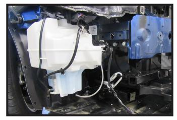
Reinstall the windshield washer fluid reservoir on the passenger side of the vehicle.
