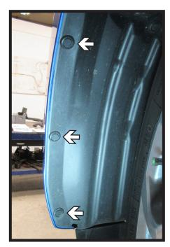
3. Remove the three (3) push pins in front of the tire in the wheel well. Do this on both sides of the vehicle.
