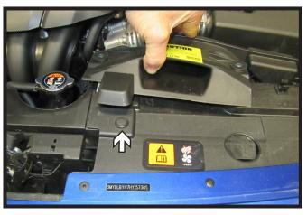
2. Lift up the plastic piece on the driver side of the vehicle and remove the one (1) push pin.
