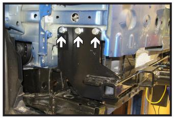
14. Insert three (3) 3/8" bolts with lock washer and whiz nuts into the side plate of the baseplate. Do this on both sides of the vehicle.
