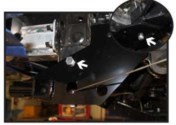
10. Install the spacer tube thru the frame on the driver side. Position the DS baseplate onto the frame and install the 1/2" x 4" bolt and hardware. Do not fully tighten.
