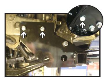
9. Using a 1/2" drill bit, ream the lower existing hole thru the frame. Install the 1/2" hardware and fully tighten the 1/2" bolt and two (2) existing bolts (inset). Using a 3/8" drill bit, drill the two (2) holes in the side plate thru the frame. Install the 3/8" hardware into the holes and fully tighten them and the 1/2" x 4" bolt.
