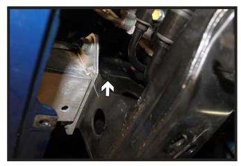
Remove the plastic frame plug for nut plate access. Do this on both sides of the vehicle.
