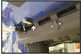
Optional Breakaway: Install the breakaway in the desired location using one of the existing lower outer valance screws.
