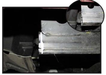
Using a reciprocating saw trim the indicated area so that it is flush with the bracket above as shown in inset. Do this on both sides of the vehicle.
