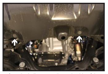
2. Using a 12MM socket, remove the four (4) screws from the belly pan on the underside of the vehicle.
