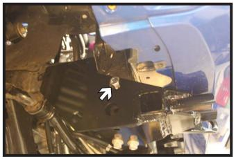
8. Slide the spacer tube into the frame. Install the 1/2" x 4" bolt thru the outside of frame with the 1/2" hardware on the inside. Do not fully tighten.
