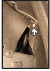
5. Loosen the wheel well liner by removing the lower screw with a 10MM socket (left) and removing the push pin in the wheel well (right). Pull back the liner to access the frame. Do this on both sides of the vehicle.
