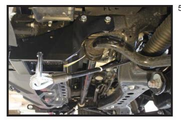
5. Attach the permanent baseplate safety cables to the provided convenience link on the baseplate. The photo shows the recommended installation of the cables to frame of vehicle. Additional options may interfere with suggested mounting; in this case, secure the cables to a solid piece of the frame as described in the instructions included with the permanent baseplate safety cables. Be sure the safety cables do not rub against any hoses or moving parts. Do this on **BOTH** sides of the vehicle.
