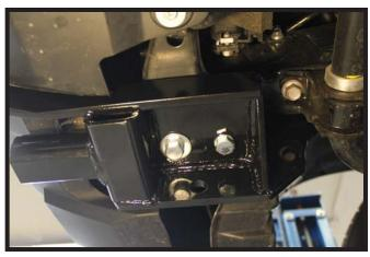
3. Install the baseplate onto the frame with the supplied 12MM hardware. Fully tighten all hardware. Do this on both sides of the vehicle.
