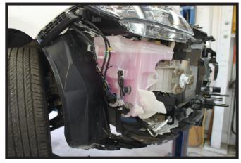
15. Trim the lower left corner of the washer reservoir as shown (left). Reinstall the washer reservoir to the vehicle.
