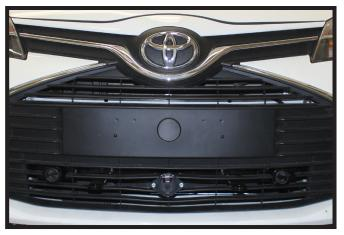
19. Hold the fascia as close to its original position, mark and trim the fascia around the convenience links and attachment tabs. Reinstall the fascia.
