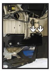
13. Install the support onto the baseplate with the 3/8" hardware (left). Do this on both sides of the baseplate. Fully tighten all hardware.
