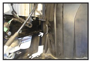
17. Notch the wheel well liner as needed around the support as shown for fascia installation. Do this on both sides of the vehicle.
