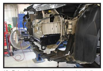
12. Reinstall the extensions/baseplate to the vehicle.
