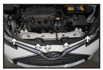
1. Remove the five (5) push pins from the top edge of the fascia.
