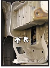
7. Using a 14MM socket, remove the four (4) bolts from the frame extension. There are two (2) on top & two (2) on the lower side. Do this on both sides of the vehicle.
