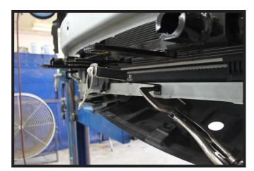
18. **Optional Breakaway:** At the desired location along the lower frame lip. Drill a 1/4" hole and install the bracket with the supplied 1/4" hardware.
