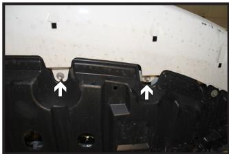
Using a 10MM socket, remove the eight (8) screws from the underside of the fascia. There are four (4) on each side.
