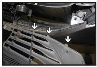
2. Unsnap the six (6) tabs from the lower grille to the fascia. There are three (3) on each side. Set the grille aside.
