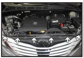
1. Remove the six (6) push pins from the top edge of the grille.
