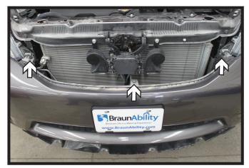
3. Remove the three (3) push pins from the top edge of the fascia.
