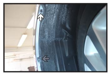
4. Using a Phillips screwdriver, remove the screw from the upper outer edge of the wheel well (white). Then turn the lower pin 1/4 turn to release the fascia from the wheel well liner (gray). Do this on both sides of the vehicle.
