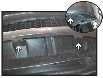
5. Using a 10MM or Phillips, remove the eight (8) screws from the underside of the fascia. There are four (4) on each side. Pull the corners of the fascia away from the vehicle disconnecting any electrical connections and set the fascia aside.
