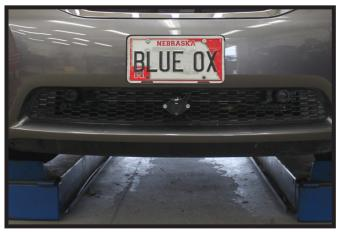
13. Hold the fascia as close to its original position, mark and trim the fascia around the convenience links and attachment tabs. Reinstall the bumper, fascia and grille.
