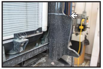
8. Trim the plastic shielding on both sides of the vehicle flush with the flat spot as shown.
