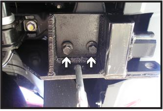
Loosely install the baseplate onto the frame using the appropriate hardware for your model into the existing tow hook holes. Do this on both sides of the vehicle.
