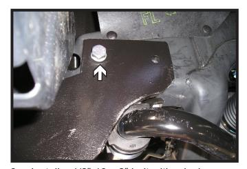
3. Install a 1/2"-13 x 2" bolt with a lock washer into the existing hole and a 1/2" nut plate on the inside of the frame. Do this on both sides of the vehicle. Fully tighten the 1/2" bolts and tow hook bolts.
