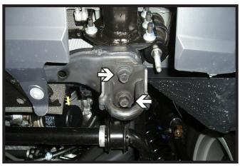
Using a 17MM socket, remove the two (2) bolts from the tow hook. Do this on both sides of the vehicle. The tow hooks will not be reinstalled.
