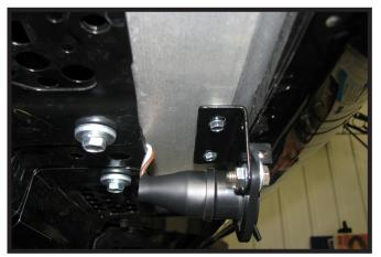
Attach the electrical bracket to the lower fascia with the supplied screws, using washers in between the bracket and fascia
