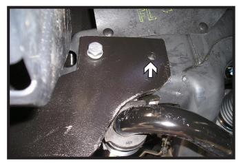
4. Using a 17/32" drill bit, drill the rear hole thru the frame. Install a 1/2"-13 x 2" bolt with a lock washer into the existing hole and a 1/2" nut plate on the inside of the frame. Do this on both sides of the vehicle. Fully tighten all hardware.
