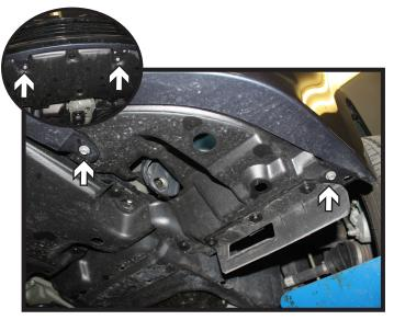
Using a 10MM socket, remove the six (6) screws from the underside of the fascia. There are two (2) on each corner and two (2) in the middle. Carefully remove the fascia from the vehicle, disconnecting all electrical connections and set the fascia aside.
