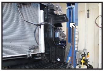
6. Unsnap the plastic shroud from the vehicle and set aside. Do this on both sides of the vehicle.
