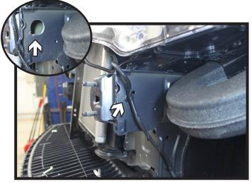
Disconnect the electrical line on the side of the frame. Using a 1-1/4" hole saw, drill an access hole as shown for nut plate installation (inset). Do this on both sides of the vehicle.
