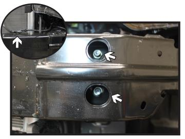
5. Disconnect the electrical line on the top side of the bumper (inset). Using a 14MM socket, remove the four (4) nuts from the bumper. There are two (2) on each side and set the bumper aside.
