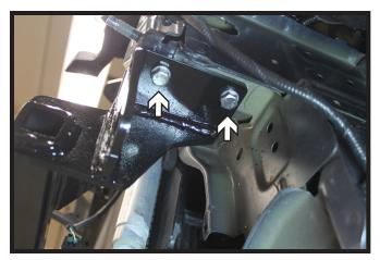
9. Using a 13/32" drill bit, drill the four (4) holes thru the frame on the underside of the baseplate. There are two (2) on each side. Install 3/8"-16 x 1-1/4" bolts with 3/8" lock washers into the existing frame holes and secure with 3/8"-16 nut plates on the inside of the frame. Fully tighten all fasteners.
