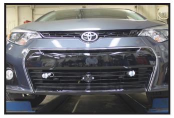
11. Hold the fascia as close to its original position, mark and trim the fascia around the convenience links and attachment tabs. Reinstall the bumper, styrofoam support and fascia.
