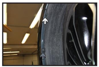
Turn the lower pin 90° to release (gray). Then remove the push pin above (white). Do this on both sides of the vehicle.
