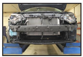
4. Remove the styrofoam support from the bumper and set aside.
