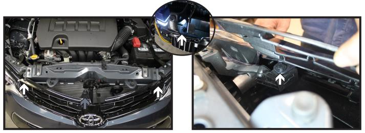
1. Using a 10MM socket, remove the screw from center top edge of the fascia (gray-left). Then remove the two (2) push pins on the outer corners (white-left). Remove the one (1) push pin from under the center bolt (white-inset). Gently pull the grille forward to expose the two (2) push pins underneath that are just below the outer corner push pins and remove (white-right).
