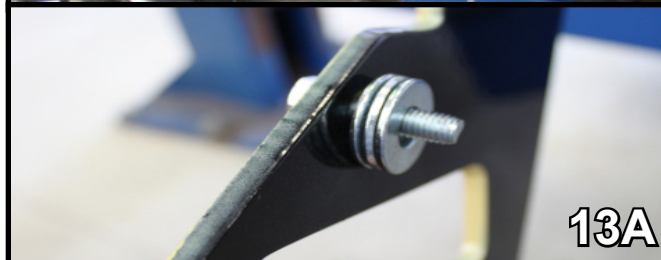
13. To install the side plate, place it over the baseplate and use a 8MM-1.25 x 30MM hex bolt with a lock washer on the outside and three flat washers with a 8MM hex nut on the inside (A, white arrow). Secure this bolt first using a 13MM socket, then use a 12MM-1.25 x 45MM hex bolt with a lock washer and a flat washer on the outside with 2 flat washers and a 12MM hex nut on the inside (B, white arrow). Tighten this bolt using a 19MM socket with Loctite Red, then remove the 8MM bolt and place it through the hose bracket and back into the hole with the lock washer on the outside and three flat washers with a 8MM hex nut on the inside. Do this on both sides of the vehicle. Replace the three 14MM bolts from step 12 after both other bolts are in place. Tighten all bolts with Loctite red.
