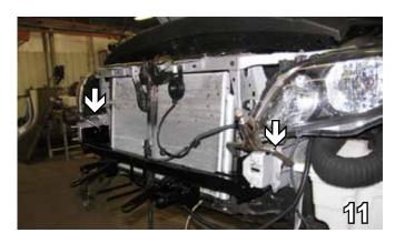
11. Slide the baseplate up between the frame rails, align with the existing hole on each side and clamp.
