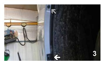
3. Just forward the front tire on the upper corner of the fascia and inside the wheel well, turn the screw 90° to remove it (white arrow). Using a flat screw driver, remove the upper push pin (gray arrow). Do this on both sides and set aside for later reinstallation.
