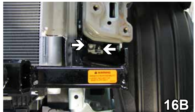
16. Reinstall the frame extension with two bolts on the top and two on the bottom. Do this on both sides.
