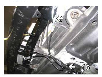
15.Attach baseplate safety cables as in above photos or as close to as possible. If you are unable to place safety cables in this location, position the cables around a solid piece of the frame.
