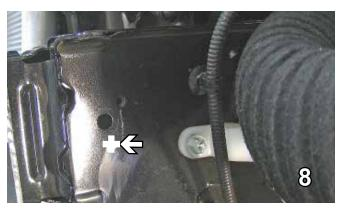
Drill a hole in the frame rail under but connected with the existing hole using the 1 1/4" hole saw on both sides. This hole will allow the installer to insert the nut plates inside of the frame rail.
