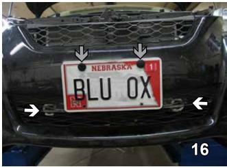
16. Hold the fascia as close to its original position as possible, mark and trim the grill with a utility knife to allow the baseplate receivers to come through (white arrows). Reinstall the fascia. The two license plate screws on the top may have to be raised up about 1/2" (gray arrows).
