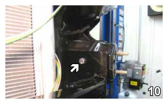
10. Insert 3/8-16 x 1 1/4" hex bolts with 3/8" lock washers attached to 3/8-16 nut plates with 14" wire inserted into the frame rail on both sides to hold the baseplate in place.
