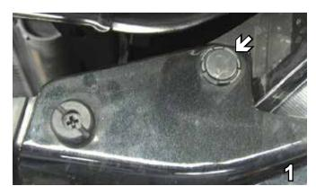
Remove push pins (white arrow) from the top corner edge of the fascia. Using the Phillips screw driver, remove the Phillips screw (gray arrow), do this to both sides and set aside for later reinstallation.
