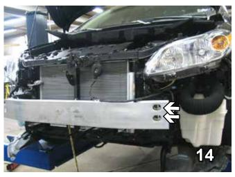
14. Reinstall the bumper. Be sure to reattach the wire loom to the top of the bumper.
