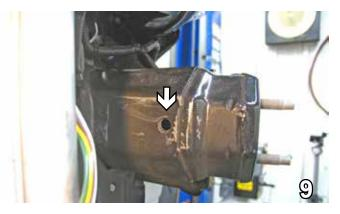
Slide the baseplate up between the frame rails and align with the existing hole on each side.
