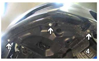
4. Just forward of the front tire underneath the bumper, using a 10MM socket, remove the three metric bolts. Do this on both sides and set aside bolts for later reinstallation.
