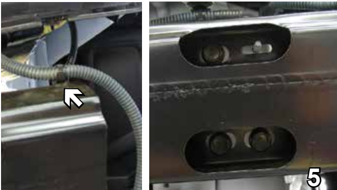
5. Pull the styrofoam off, unclip the four clips across the top of the metal bumper. Remove the bolts with a 14MM socket from both sides. Set aside for later reinstallation.
