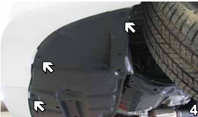
4. Using 10MM socket, remove seven metric bolts underneath the fascia.
