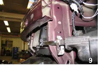
Using the reciprocating saw, cut and remove front webbing of tie down bracket, both sides. This will open area to allow baseplate to slide onto the outside of tie down bracket and frame.
