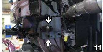
11. Slide the baseplate into place lining up and centering the holes of the baseplate with the air bag sensor holes. Insert and tighten sensor bolts to hold baseplate in place.
