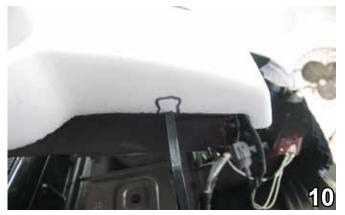
10. Align styrofoam to original position. You will need to cut out a 1/2" to 3/4" section with utility knife; do on both sides to slide back on completely.
