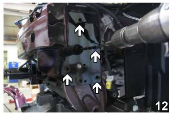
12. Using the baseplate as a template, drill the holes into the frame and webbing with the 13/32" drill bit, both sides.
