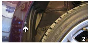
2. Using a 10MM socket, remove one metric bolt just forward of the front tire, on wheel well. Repeat for both sides of the vehicle. Set bolts aside to be reinstalled later.
