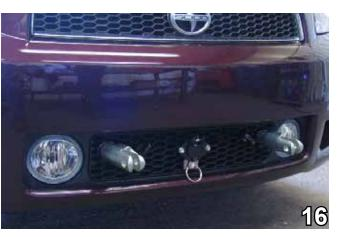
16. Reattach air dam. Align the fascia to its original position and using a side cutters, remove area around attachment tab receiver and quick link to allow it to come through the fascia. Do this to both sides of the vehicle.
