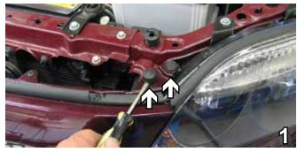
1. Using a flat screwdriver, remove one plastic push pin from both sides and one from the center. Remove hood stop push pin with the flat screw driver, both sides. Set push pins and bolts aside to be reinstalled later.
