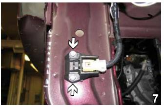
7. Using a 10MM socket, remove two metric bolts from air bag sensor. Set aside bolts and air bag sensor for later reinstallation.
