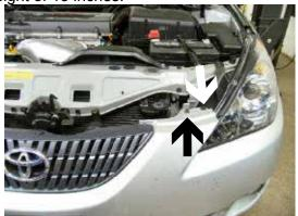
1. Remove metric bolt (Black arrow) with the 10MM socket, on both sides, and three push pins (White arrow) on top side of fascia.
