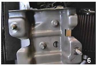
**6.** Remove two metric bolts from bumper bracket, both sides, pull forward and set aside.
