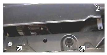
2. Remove two metric bolts from top edge of fascia's tabs with the 10MM socket. Remove one push pin.
