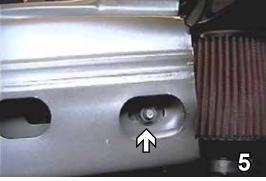
**5.** Using the 12MM socket, remove four metric bolts from metal bumper, pull metal bumper forward and set aside.
