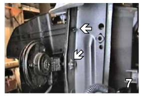
7. Pinch clips together on the back of radiator support and pull air dam forward, both sides and set aside.
