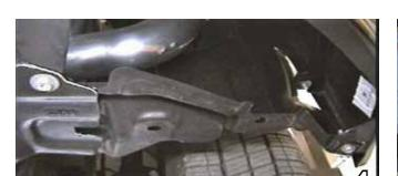
**4.** Forward of front tires on lower fascia's edge are eight metric bolts to remove with the 10MM socket.
