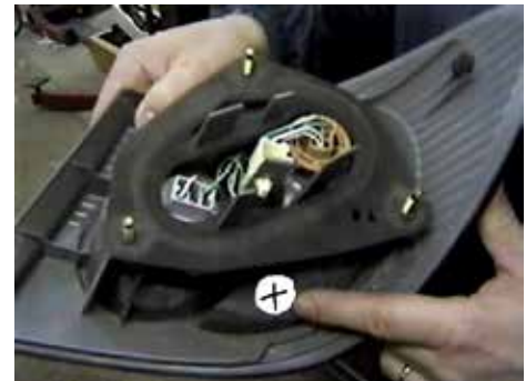
Location of the BX8869, on the bottom of the driver's side tail light assembly.
