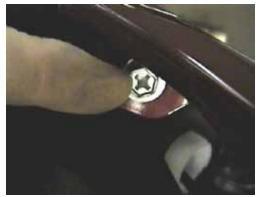
**3.** Just forward of front tire, inside wheel well, remove metric bolt with the 10MM socket, both sides.
