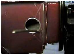
**5.** Drill 1 1/4" hole on the outside of frame end, just back from seam (see photo for general location), using the 1 1/4" hole saw.
