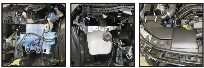
24. Reinstall windshield washer reservoir, horn, filter and sub-tank, and cover.
