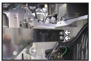
Remove the two (2) bolts on the side of the baseplate, one at a time. Apply Loctite<sup>®</sup> Red and tighten to appropriate torque. Do this on both sides of the vehicle.
