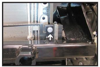
22. Insert one (1) 1/4" bolt with washer and nylon lock nut as indicated. Do this on both sides of the vehicle.
