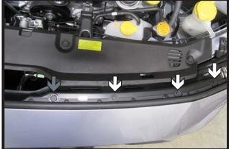
1. Using a 10MM socket, remove the four (4) bolts (white) from the top edge of the fascia. Then remove the two (2) push pins (gray).
