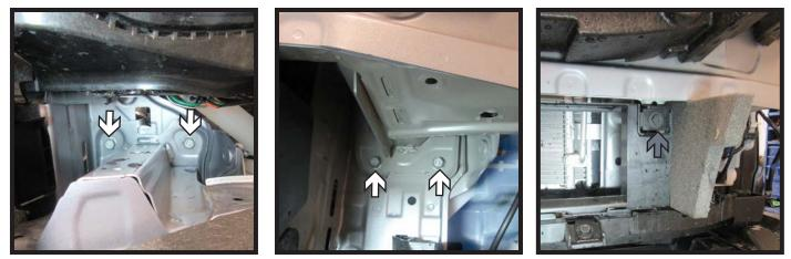
6. Using a 12MM socket, remove the four (4) bolts (white) from the bumper as indicated. Then using a 10MM socket remove the one (1) bolt (gray). Do this on both sides of the vehicle. Remove bumper, it will not be reinstalled later.
