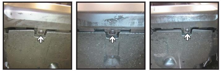
4. Using a Phillips screw driver remove the three (3) plastic screws from the underside of the fascia.
