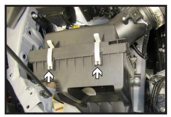
11. On the passenger side of the vehicle unsnap the two (2) clips from the top of the air filter.
