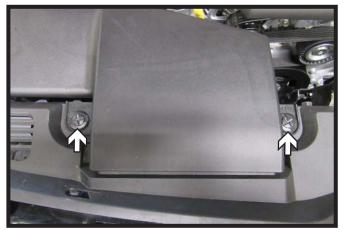
Using a flat head screw driver turn top two (2) screws 1/4 of a turn and remove plastic piece from the passenger side of the vehicle, to be reinstalled later.
