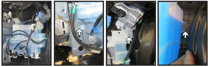
9. Unplug all of the fluid lines from the windshield washer reservoir. Then using a 10MM socket, remove the three (3) bolts holding the reservoir in place. Remove and set aside to be reinstalled later.
