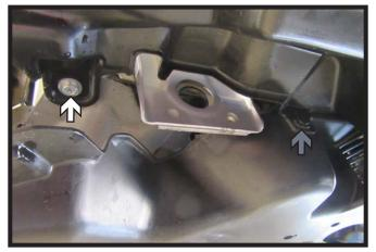
7. Pull down the belly pan and using a 10MM socket remove the one (1) bolt (white) as indicated. Then remove the one (1) push pin (gray). Do this on both sides of the vehicle.
