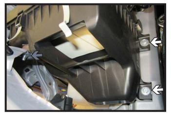
Using a 10MM socket remove the two
