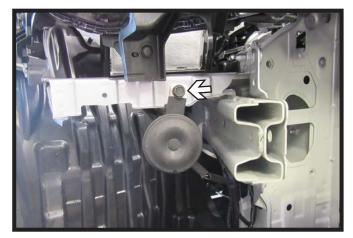
Using a 12MM socket remove the one (1) bolt holding the horn on the passenger side of the vehicle. Remove and set aside to be reinstalled later.
