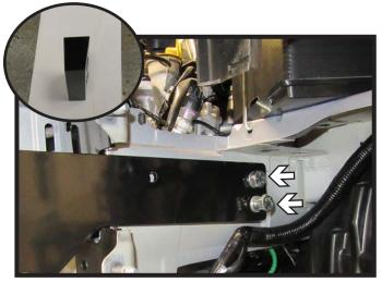
18. Slide the baseplate onto the frame. Insert wedge piece (inset) between the frame and the baseplate with the narrow edge towards the front and the wide edge towards the back. Once the wedge is in place start the two (2) 12MM bolts with lock washers. Tighten but do not use Loctite<sup>®</sup> Red at this time. Do this on both sides of the vehicle.
