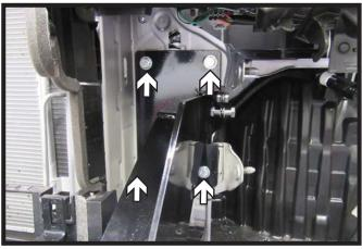
19. Insert the four (4) 8MM bolts with flat washer and lock washer into the front of the baseplate. Do this on both sides of the vehicle.
