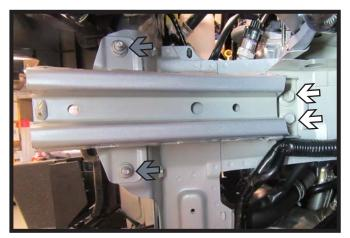
14. Using a 13MM socket remove the two(2) bolts (white) and two (2) nuts (gray) as indicated. Do this on both sides of the vehicle.
