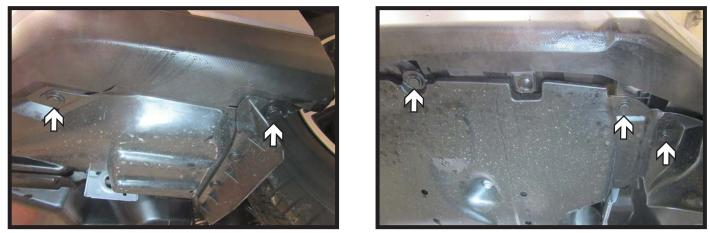
3. Remove five (5) push pins from the underside of the fascia. Do this on both sides of the vehicle.
