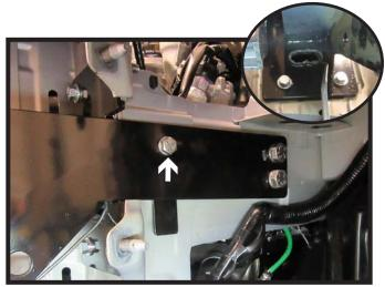
21. Start one (1) 3/8" bolt with lock washer and insert 3/8" nut plate with 14" wire through access hole on the bottom side of the baseplate (inset) and attach to back side of bolt. Then place flat spacer plate between baseplate and frame. Do this on both sides of the vehicle.
