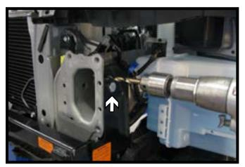
Tip the baseplate into position. Install 1/2"-13 x 1-1/4" bolts, 1/2" flat & lock washers and 1/2" lock nuts into the existing frame holes. Level the baseplate and tighten down the bolts.
