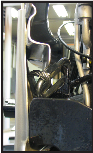
30. Attach the permanent baseplate safety cables to the provided convenience link on the baseplate. The photo above shows the recommended installation of the cables to frame of vehicle. Additional options may interfere with suggested mounting; in this case secure the cables to a solid piece of the frame as described in the instructions included with the permanent baseplate safety cables. Be sure the safety cables do not rub against any hoses or moving parts. Do this to both sides of the vehicle.
