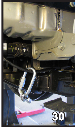
30. Attach the permanent baseplate safety cables to the provided convenience link on the baseplate. The photo above shows the recommended installation of the cables to frame of vehicle. Additional options may interfere with suggested mounting; in this case secure the cables to a solid piece of the frame as described in the instructions included with the permanent baseplate safety cables. Be sure the safety cables do not rub against any hoses or moving parts. Do this to both sides of the vehicle.
