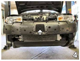
Remove one pushpin from the Styrofoam bumper. Set Styrofoam bumper and pushpin aside to be reinstalled later.
