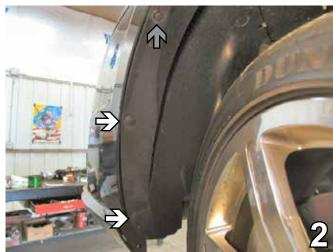
Inside the wheel well, just forward of the front tire, use a 7MM socket to remove one metric bolt, as indicated by the grey arrow in the photo above. Remove two pushpins, as indicated by the white arrows in the photo above. Set bolt and pushpins aside to be reinstalled later. Do this to both sides of the vehicle.
