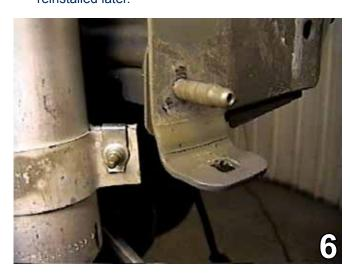
6. Bend the upper fascia support bracket forward 90 degrees. Do this to both sides of the vehicle.
