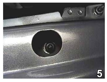
5. Using the 13MM socket, remove six metric bolts from the metal bumper. Pull it forward and set it aside to be reinstalled later.
