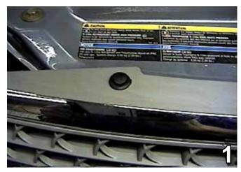
Remove three pushpins from the top side of the grille. Set the pushpins and the grille aside to be reinstalled later.
