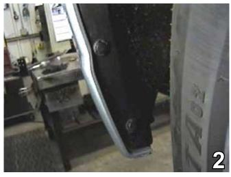
2. Just forward of the front tires, in the wheel well, remove four pushpins. Set the pushpins aside to be reinstalled later. Do this to both sides of the vehicle.
