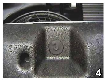
4. Just forward of the wheel well, behind the fascia's upper corner, push clip up to unlock the fascia. Do this to both sides of the vehicle. Fascia will unlock properly when you hear a click, pull the fascia forward and set it aside to be reinstalled later. Remove three pushpins from the Styrofoam insert. Pull the Styrofoam bumper forward. Set the pushpins and the Styrofoam bumper aside to be reinstalled later.
