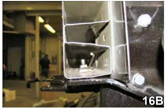
16. Using the baseplate as a template, drill a hole into the bottom of metal bumper with the 13/32" drill bit, both sides. Insert the 3/8" nut plate with the 12" wire into the open end of metal bumper to align with drilled hole, tighten 3/8-16 x 1 1/2" hex bolt and lock washer with the 9/16" socket, both sides. Be sure and use loctite red on all bolts before tightening. Tighten all bolts according to torque chart in the General Instruction sheet.
