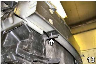
13. Using the utility knife, cut and remove the small tab of air dam just below metal bumper. This will open area for baseplate install.
