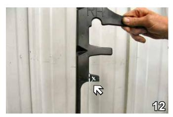
12. Using the utility knife, cut and remove the small tab of air dam and reinstall both sides. This will open area just below metal bumper for baseplate install.
