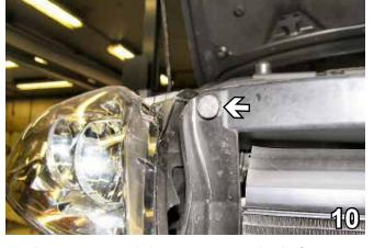
10. Remove one christmas tree push pin from upper air dam, just inside headlight assembly, both sides.
