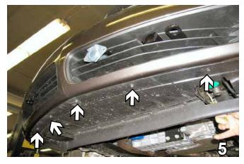
5. Remove the five metric bolts from lower edge of fascia with the 7MM socket, pull corners of fascia to the side of vehicle to release tabs, pull fascia forward and set aside.
