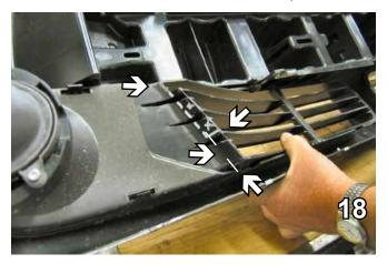
18. Lay fascia face down on a soft surface, so as not to scratch, using the utility knife, cut and remove 1/2" of the outer edge of fascia's opening, both sides.
