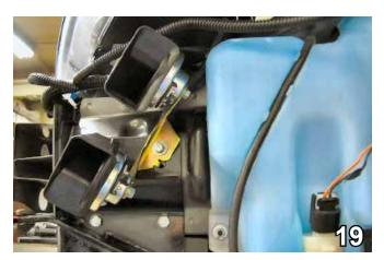
19. Remove horn bracket's existing metric bolt on the driver's side from baseplate (installed in step 15). Reinstall horn bracket using the 6MM-1 x 30MM, 6MM lock washer and 1/4" flat washer.
