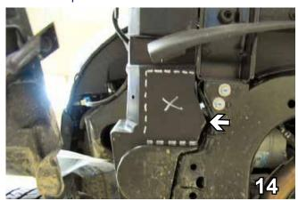
14. Cut opening on lower belly pan to gain access to the bottom of frame rail opening for nut plate insertion, both sides (Passenger's side is shown in photo).
