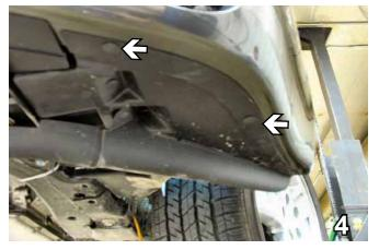
Remove the two push pins on lower edge of fascia, just forward of the front tire, both sides.
