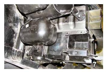
7. Remove the two push pins from the bottom and front of air baffle and one metric bolt from between the wheel well and baffle using the 10MM socket.
