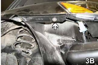
3 .Using the 10MM socket, remove the back metric bolt from corner of fascia, just above front tire (left photo) and loosen the front metric bolt on the inside of wheel well, both sides (right photo showns passenger's side location with fascia off).
