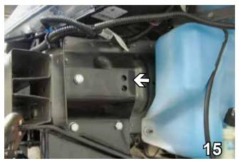
15. Slide baseplate onto the frame rail and up to bottom of metal bumper, clamp baseplate to bumper with vise grip, both sides. Align baseplate to existing bolt location for the horn bracket on the driver's side, replace and tighten existing metric bolt for horn bracket to hold baseplate in place. Be sure to align lower holes of baseplate to the center of lower frame webbing before drilling holes. Align passenger's side of baseplate to the frame to the same location as the driver's side and
