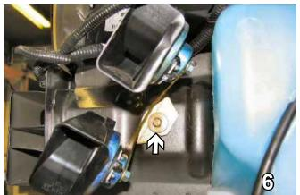
6. Using the 10MM socket, remove metric bolt from horn bracket on the driver's side and set assembly aside.
