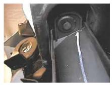
**8.** Remove push pin from belly pan, both sides. Pull belly pan forward and set aside.
