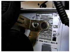
**6.** Using the 10MM socket, remove the metric bolt from horn bracket, unplug and set aside.
