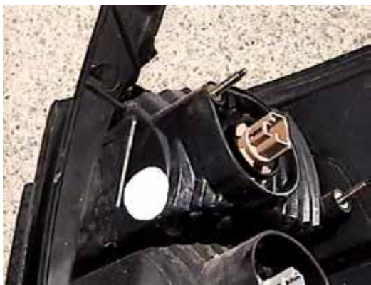
Location of the BX8869 (Photo of driver's side taillight assembly)
