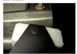
5. Just forward of lower air dam, on the back side of fascia, are four push pins to remove. Pull fascia forward and set aside.
