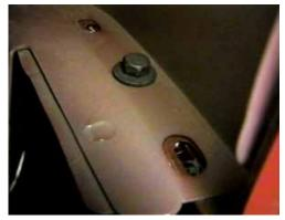
**4.** Using the 10MM socket, remove two metric bolts on fascia corner inside wheel well, both sides.
