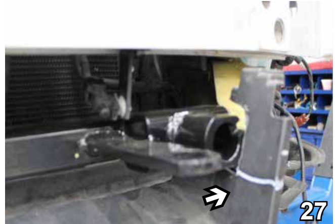
27. Reinstall plastic belly pan under metal bumper, under baseplate. In order to accommodate attachment tabs, trim belly pan tabs parallel with the ground as marked in the above photo. Do this on both sides. (NOTE: Fascia will hold the belly pan in place when it is reinstalled.)
