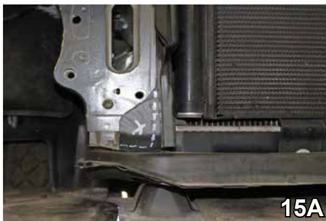
15. With reciprocating saw, on the passenger's side only, trim metal next to radiator flush with the front of the bracket (15A). After trimming is completed, tap remaining piece toward radiator to make flush and allow for baseplate mounting (approximately 1/4") (15B).
