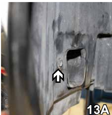
13. To remove the air baffles, with a 10MM socket, in front of the tire, remove bolt (13A), under the air baffle, remove 2 bolts (13B) and unsnap the air baffle at the bottom of the metal bumper (13C). Do this on both sides. Pull down air baffles to remove and set aside air baffles and bolts to be reinstalled later.
