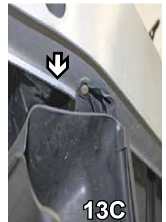
13. To remove the air baffles, with a 10MM socket, in front of the tire, remove bolt (13A), under the air baffle, remove 2 bolts (13B) and unsnap the air baffle at the bottom of the metal bumper (13C). Do this on both sides. Pull down air baffles to remove and set aside air baffles and bolts to be reinstalled later.
