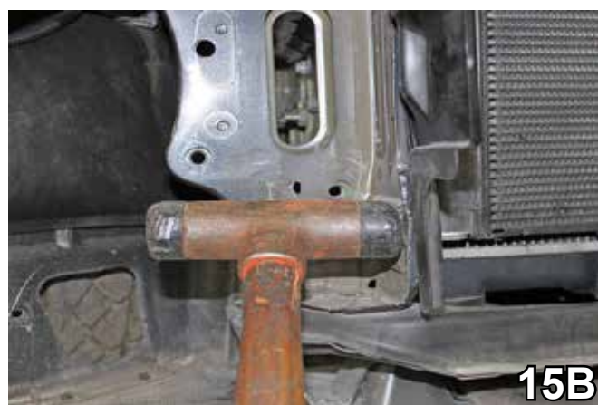
15. With reciprocating saw, on the passenger's side only, trim metal next to radiator flush with the front of the bracket (15A). After trimming is completed, tap remaining piece toward radiator to make flush and allow for baseplate mounting (approximately 1/4") (15B).
