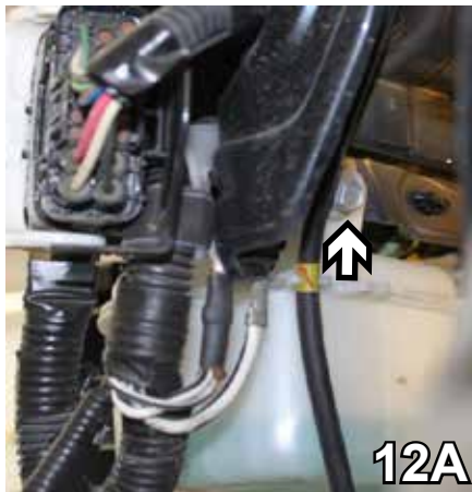
12. To remove washer fluid reservoir, with a 10MM socket, remove bolt in back (12A), in front and to the left of the reservoir (12B) as well as on the topside of the reservoir just above headlight (12C). Disconnect electrical, and plug fluid lines and set aside to be reinstalled later. NOTE: Two of the Three existing bolts will be replaced with bolts provided (12A and 12B).
