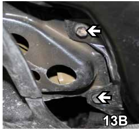
13. To remove the air baffles, with a 10MM socket, in front of the tire, remove bolt (13A), under the air baffle, remove 2 bolts (13B) and unsnap the air baffle at the bottom of the metal bumper (13C). Do this on both sides. Pull down air baffles to remove and set aside air baffles and bolts to be reinstalled later.
