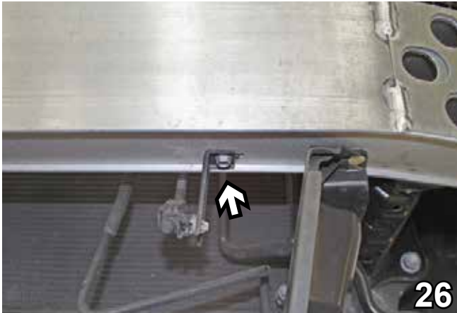
26. Reinstall metal bumper. Remount the temperature sensor bracket and reattach sensor to the bracket. Use existing bolts.
