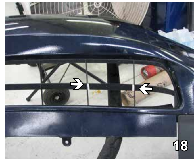
18. Trim the fascia. Using a utility knife, remove the second horizontal style from the end. Do the same on the other side.
