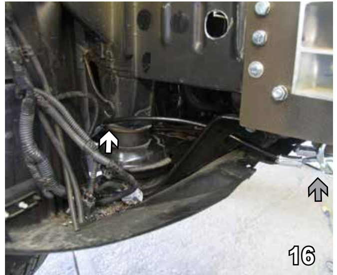
16. Attach the permanent baseplate safety cables to the provided convenience link on the baseplate (see grey arrow). The photo above shows the recommended installation of the cables to frame of vehicle (see white arrow). Additional options may interfere with suggested mounting; in this case secure the cables to a solid piece of the frame as described in the instructions included with the permanent baseplate safety cables. Be sure the safety cables do not rub against any hoses or moving parts. Do this to both sides of the vehicle.
