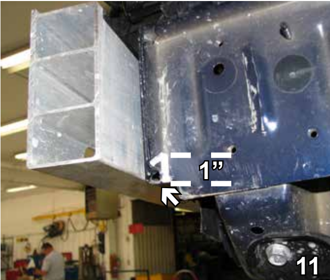
11. Behind the bumper, cut out a notch. Cut up one inch then slant down to the corner. Do this on both sides of the vehicle.
