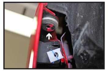
3. Using a T30 Torx, remove the screw from behind the wheel well cover where the fascia meets the fender. Repeat on the other side of the vehicle.
