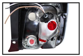
11. Possible location for the BX8869: Using a 20 Torx remove the four (4) screws from the back plate and remove (Right). Using a 1" hole saw drill a hole into the metal portion of the light as shown. Put the wires thru and silicone around the hole to seal.
