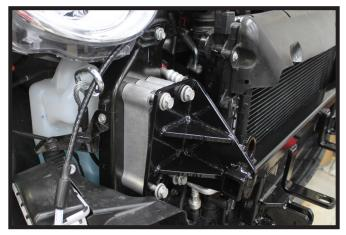
Install the baseplate onto the vehicle, using the existing spacer and 10MM bolts. Repeat on the other side of the vehicle. Tighten down baseplate to the vehicle.
