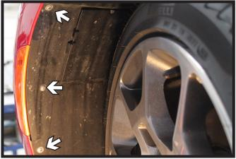
2. Using a phillips screwdriver, remove the three (3) screws from the wheel well in front of the tire. Repeat on the other side of the vehicle.
