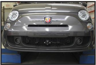
Hold the fascia up to the vehicle as close to it's original position. Mark and trim with a utility knife until the fascia is clear of the attachment tabs and convienence links. Reinstall the fascia.
