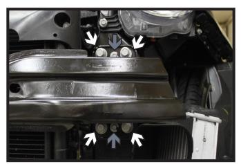
Using a 15MM socket, remove the four (4) larger bolts from bumper (white). Then using a 10MM socket, remove the two (2) smaller bolts (gray). Repeat on the other side of the vehicle. The metal bumper and smaller bolts will not be reused.
