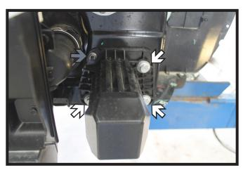
5. On the bumper horn, using a 15MM socket, remove the three (3) bolts (white). Then using a 10MM socket, remove the one (1) nut. Do this on both sides of the vehicle. The bumper horns will not be reinstalled, but the existing bolts will be reused.
