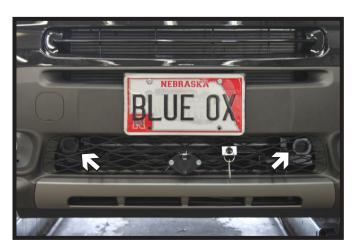
14. Hold the fascia as close to its original position, mark and trim the fascia around the convenience links and attachment tabs. Reinstall the fascia.
