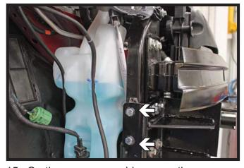
15. On the passenger side, move the windshield washer reservoir to the side. Insert 3/8"-16 x 1" bolts attach to 3/8"-16 nylock nuts. Reattach the washer reservoir. Use the same bolts and nuts on the driver side.
