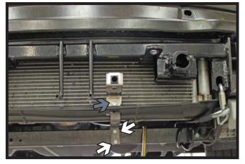
18. **Optional (continued from #17):** Attach the bracket to the lower frame with two (2) #10-16 x 1" self drilling screws (white arrows). Attach the breakaway to the bracket with 1/4"-20 x 3/4" hex bolt and 1/4"-20 hex nut (gray arrow).
