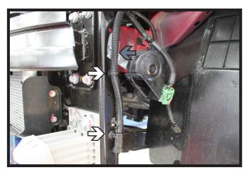
On the driver side, remove the two (2) clips from the frame (white). Using a 10MM socket remove the bolt from the horn bracket (gray) and unplug the wiring.
