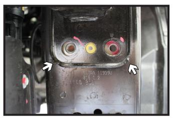
11. Using a hammer, flatten the tips on the corners of the bumper bracket. Do this on both sides.
