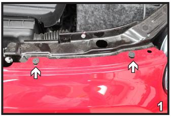
1. Using a T30 Torx, remove the four (4) screws from the top edge of the fascia. There are two (2) on each side.
