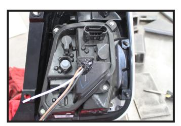
22. Using a 1/2" drill bit, drill a hole in the triangle part of the back piece. Put the wires through the hole and silicon around it. Reinstall the screws. Do this to both sides of the vehicle.
