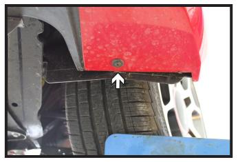
Using a phillips screwdriver, remove the one (1) screw from the bottom corner of the fascia. Do this on both sides of the vehicle.
