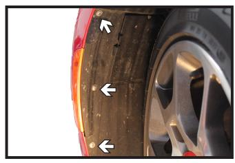
2. Using a phillips screwdriver, remove the three (3) screws from the wheel well. Do this on both sides of the vehicle.
