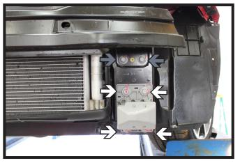
10. Using a 14MM socket, remove the four (4) bolts holding the fascia guard (white arrows). Cut the upper mounting holes off the fascia guard, flush with the top surface of the fascia guard. Reinstall the fascia guarding using only the bottom two (2) bolts. Using a 15MM socket, remove the two (2) bolts under the bumper (gray arrows). These bolts will not be reinstalled. Do this to both sides.
