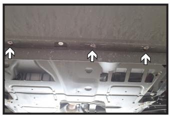
5. Using a T30 Torx, remove the three (3) screws from the bottom edge of the fascia. DO NOT remove the silver screw.
