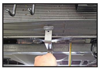
17. **Optional:** Center the breakaway bracket between the electrical rod and the convenience link and mark the plastic guard. Cut the hole for the bracket to go through with a utility knife.
