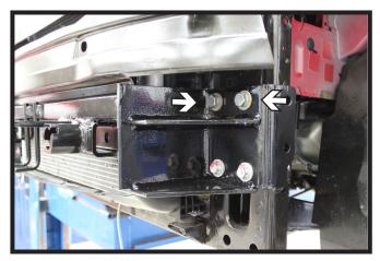
13. Slide the baseplate in place, aligning with the existing holes in the end of the frame mount. Reinstall the existing bolts in the bottom two (2)holes. In the top two (2) holes, insert 10MM-1.25 x 40MM hex bolts, 10MM lock washers and 3/8" flat washers. Do this on both sides.
