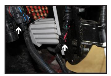
7. Unplug the two (2) connectors for the lights in the fascia, by releasing the clip on the bottom side of the plugs. Do this on both sides of the vehicle.
