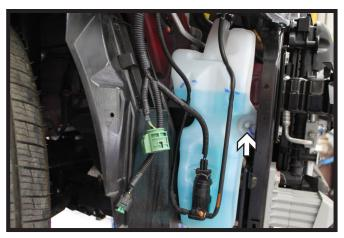
Using a 10MM socket, loosen the bolt on the right hand side of the washer reservoir.
