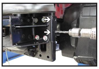
14. Using the baseplate as a template with a 13/32" drill bit, drill the two (2) side holes. Do this on both sides.
