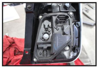
20. On the backside of the tail light, using a T20 Torx remove the four (4) screws. Remove the back piece. Do this on both sides.
