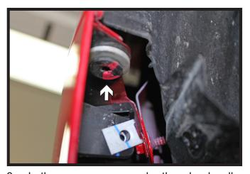
In the upper corner, under the wheel well cover, remove the one (1) screw with a T30 torx. Do this on both sides of the vehicle.
