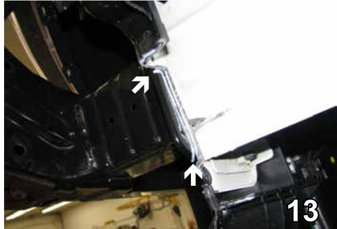
13. Temporarily put the bumper back on to mark on the back side the area to be trimmed. Remove this area with the reciprocating saw, both sides.
