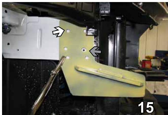
15. Slide the baseplate on to the frame rail to align with the existing hole for the washer reservoir on the passenger's side (gray arrow). Be sure the baseplate is level with respect to the vehicle frame. Clamp the baseplate to the frame rail with the vise grip. Using the baseplate as a template, drill the top inside hole with the 13/32" drill bit (white arrow).
