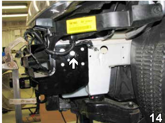
14. Insert 3/8-16 x 1 1/4" bolt with 3/8" lock washer and fasten to 3/8-16 nut plate inserted into the 1 1/4" hole. Be sure to use loctite on this bolt. Drill the other three holes. Remove the 6MM bolts, inserted in step 12. Do this on both sides of the vehicle.
