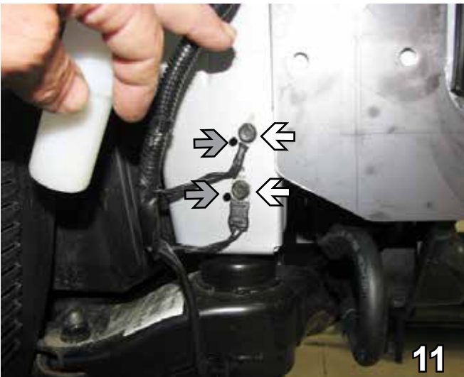
11. Loosen the ground wires (white arrows). Flatten the pins (gray arrows) and turn the wires to a vertical position. Do this on both sides of the vehicle.
