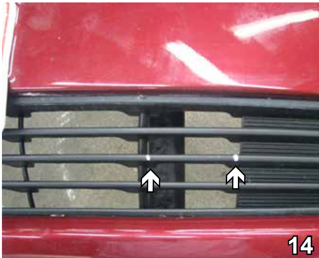
14. Align fascia to its original position, cut the center rib out as needed on the far end of the fascia grille using a hack saw blade. This will allow for the attachment tab receiver to come through. Do this on both sides of the vehicle.
