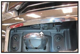
On the passenger side of the vehicle pull the indicated plug through the backside of the fascia and let hang.
