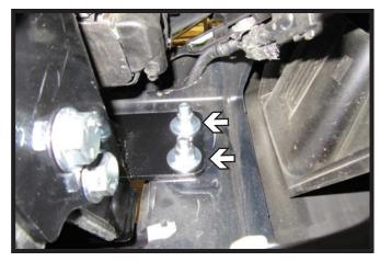
17. Insert two (2) 1/2" x 2" bolts with a flat washer and nylon lock nut on the back side to attach the convenience link. Do this on both sides of the vehicle.
