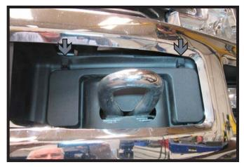
Remove the two (2) clips from each side above the tow hook. Do this on both sides of the vehicle.
