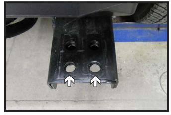
Before installing the baseplate use a 11/16" drill bit to drill out the front two (2) holes on the tow hook bracket. Do this on both sides of the vehicle.
