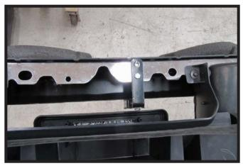
14. **Optional:** On the backside of the fascia there are two (2) existing holes above the license plate, use either hole to attach the bracket for the breakaway switch.
