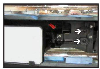
Reinstall bumper, insert the existing two
