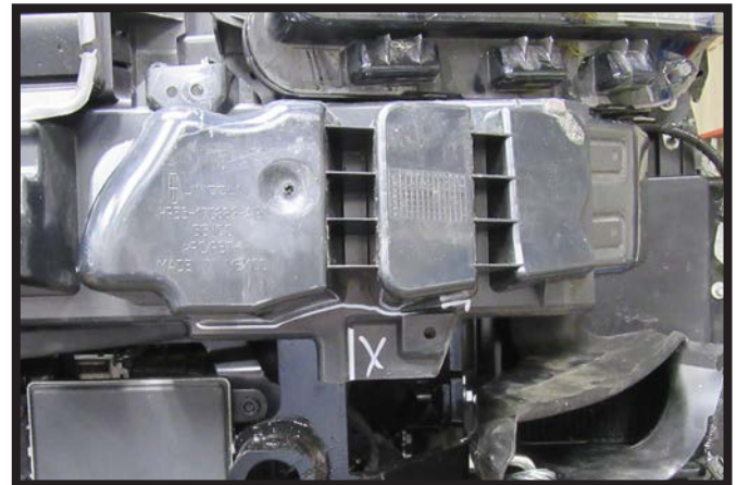
27. Hold the plastic piece and mark as shown the areas that interfere with the baseplate. Then trim indicated areas to allow to fit around baseplate. After trimmed reinstall plastic piece to the back of the fascia.
