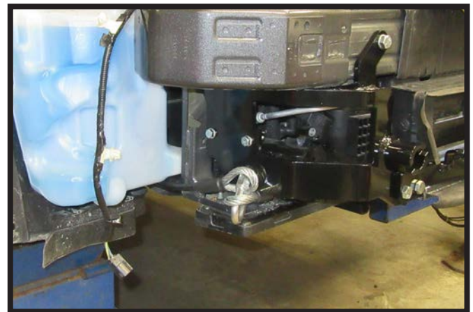
23. Attach the permanent baseplate safety cables to the provided convenience link on the baseplate. The photo above shows the recommended installation of the cables to frame of vehicle. Additional options may interfere with suggested mounting; in this case, secure the cables to a solid piece of the frame as described in the General Information sheet. Be sure the safety cables do not rub against any hoses or moving parts. Do this on BOTH sides of the vehicle.
