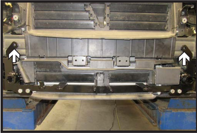
20. Using a 1/2" drill bit, drill out the top two (2) holes as indicated.
