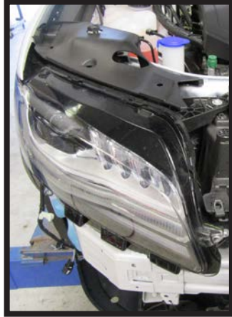
24. Reattach horn brackets (left) and headlights (right) to both sides of the vehicle.
