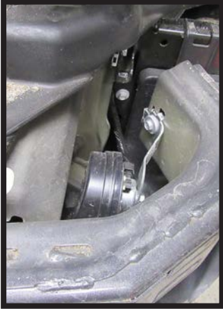
24. Reattach horn brackets (left) and headlights (right) to both sides of the vehicle.
