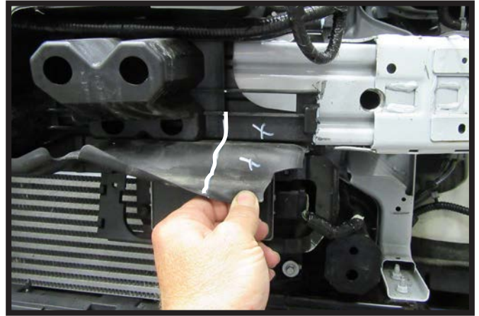
12. Using a utility knife remove the indicated area above the adaptive cruise control sensor on the driver side of the vehicle.
