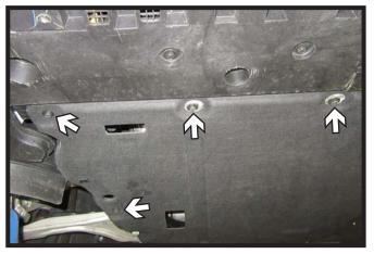
4b. Then using a 10MM socket remove the eight (8) bolts along the middle, four (4) on each side.
