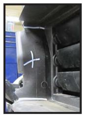
12. Using a recipricating saw remove the marked areas on both sides of the vehicle next to the shutters.
