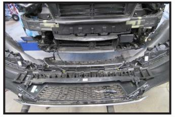
6. Pull the corners of the fascia away from the vehicle disconnecting any electrical connections and set the fascia aside.
