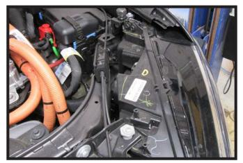
Using a T25 Torx, remove the one (1) screw from the headlight. Using a 10MM socket, remove the two (2) bolts holding the headlight in. Slide the headlight out. Do this for both sides of the vehicle.
