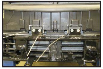
21. Using the baseplate as a template run a 3/8" drill bit through each of the four (4) holes at the top of the baseplate. Then insert the 3/8" nut plate and 3/8" x 1-1/4" lock washer.
