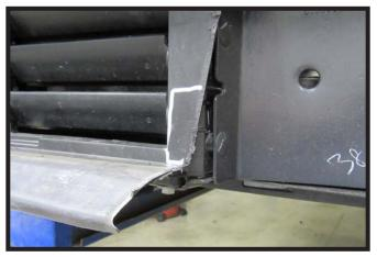
Using a recipricating saw notch and remove marked area right under the gusset to the corner and then down. Do this only on the driver's side of the vehicle.
