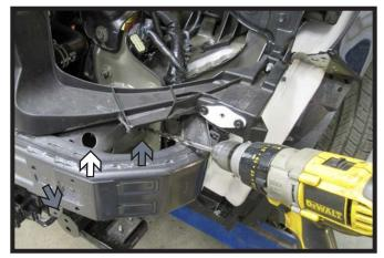
10. Using a 1-1/4" hole saw, drill access holes in the side of the frame on both sides of the vehicle as shown (white).
