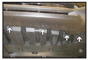
3. Underneath the car, using a 7MM socket, remove twelve (12) bolts total. There are two (2) on each side, and eight (8) on the front. (Driver's side and front pictured)
