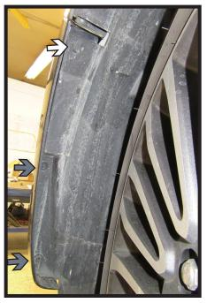
In front of the tire, in the wheel well, remove one (1) push pin (white). Using an 8MM socket, remove two (2) bolts (gray). Do this for both sides of the vehicle.
