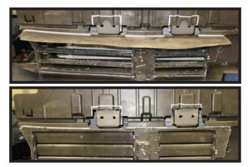
15. Using a recipricating saw remove the marked areas above the shutters. (The top picture is the before and the bottom picture is the after.)
