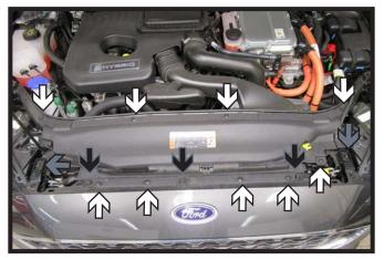
1. Remove nine (9) push pins (white) from the fascia cover. Remove fascia cover and set aside. Using a 10MM socket, remove three (3) bolts (black) from the top of the fascia, and two (2) bolts (gray) from the plastic covers.
