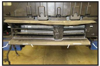
14. Using a recipricating saw follow the line as marked and remove the piece below the shutters.
