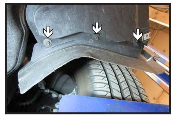
4a. Remove the belly pan. Using a 7MM socket remove the three (3) bolts in front of the tire on both sides of the vehicle.
