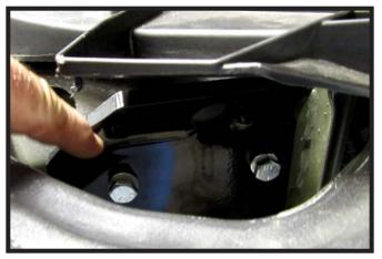
18. Slide the baseplate Into position and insure it is level and aligned with existing holes, before clamping to the frame rail on both sides with large vise grips. Insert 3/8"-16 x 1-1/2" Hex Head Bolt with 3/8" lock washer into the top two (2) pre-existing holes on both sides of the vehicle, with the 3/8" nut plate on the inside of the frame.
