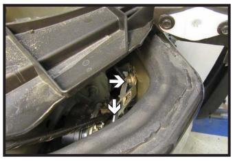
Using a 10MM socket, remove the two (2) bolts holding the horn bracket in place. Remove the horn bracket. Do this for both sides of the vehicle.
