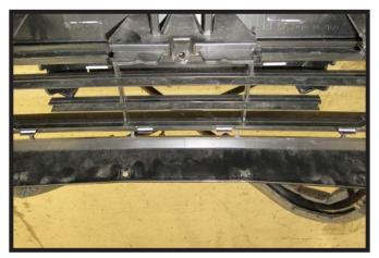
On the back side of the fascia near the bottom use a recipricating was to trim the four (4) tabs so that they are flush with the rest of the fascia.
