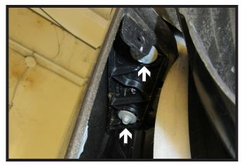
5. In front of the tire, pull back the wheel well cover. Using an 10MM socket, remove the two (2) revealed bolts. Do this for both sides of the vehicle.
