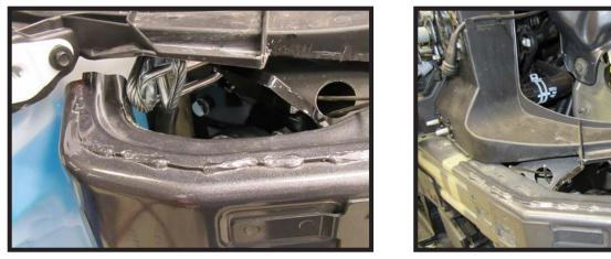
20. Attach the permanent baseplate safety cables to the provided convenience link on the baseplate. The photo above shows the recommended installation of the cables to frame of vehicle. Additional options may interfere with suggested mounting; in this case, secure the cables to a solid piece of the frame as described in the General Information sheet. Be sure the safety cables do not rub against any hoses or moving parts. Do this on **BOTH** sides of the vehicle.
