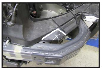
9. Using a reciprocating saw, trim the plastic shrouding approximately as shown for baseplate clearance.
