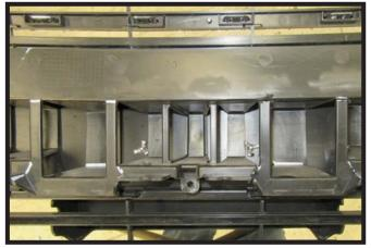
16. On the back side of the fascia use the recipricating saw to remove the pieces as marked on both sides near the center of the fascia.
