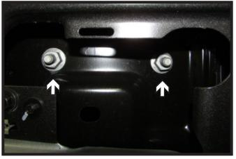
Using a 21MM socket, remove the two (2) nuts from the face of the bumper. Do this on both sides of the vehicle.
