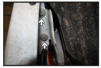
Using a 10MM socket, remove the two
