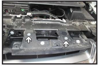
2. Using a T30 Torx, remove the four (4) screws from the top edge of the grille. There are two (2) on each side.
