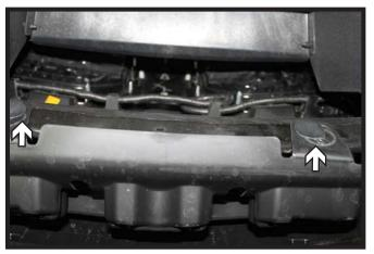
On the underside of the fascia towards the middle, remove the two (2) push pins.
