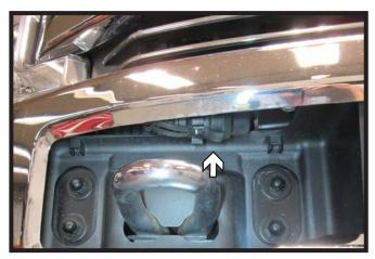
On the passenger side of the vehicle pull the indicated plug through the backside of the fascia and let hang. Pull the bumper forward and set aside to be reinstalled later.
