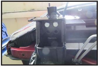
10. Slide the baseplate on, align with the existing front tow hook holes. Bolt on first using two (2) of the 5/8" x 1-3/4" bolts, and lock washers.
