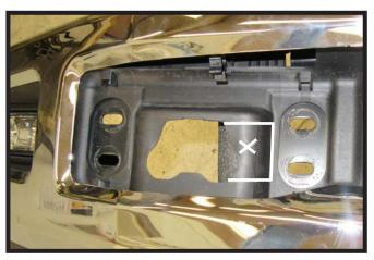
12. Using a reciprocating saw remove the marked area on both sides of the fascia towards the inside near the licence plate.
