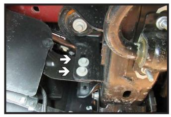
2. Behind the bumper on the frame by the headlights there are two (2) bolts that need to be removed using a 15MM socket, do this on both sides of the vehicle.
