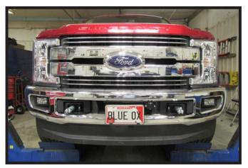
14. Reinstall bumper, bolts, and reconnect wiring.
