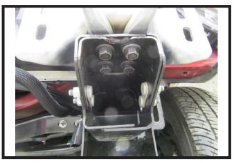
Using an 18MM socket remove the four
