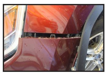
Lift up on the corners of the fascia to unsnap and pull it away from the vehicle disconnecting any electrical connections and fluid lines. Set the fascia aside.
