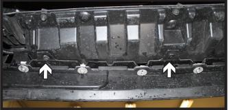
4. Using a 8MM socket, remove the seven (7) screws from the underside of the fascia. There are two (2) in each corner and three (3) across the front.
