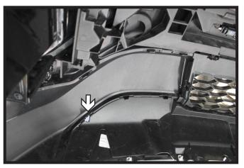
17. On the backside of the fascia trim the outer tab shown flush with the backside of the fascia for clearance of the baseplate. Do this on both sides of the vehicle.
