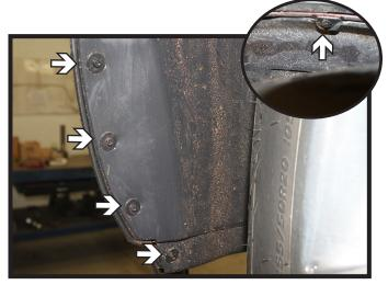
Using a 5.5MM socket, remove the seven (7) screws from the edge of the wheel well. Then above the center of the wheel, remove the push pin (inset). Do this on both sides of the vehicle.
