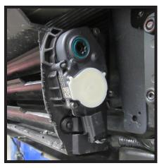
11. Using a reciprocating saw, trim the marked areas beside the shutters. On the driver side, ensure the cutting is performed against the contour of the motor.
