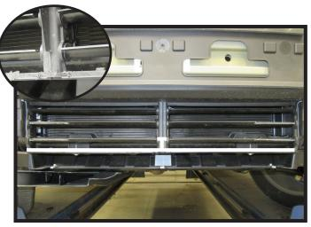
10. Using a reciprocating saw, trim the marked area to be flush with the shielding. Also, trim the middle plastic about 1-1/2" up to the bottom shutter, ensuring it is also flush with the plastic shielding.
