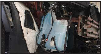
16. Install nine (9) 1/4" washers onto the two (2) studs for the washers reservoir (top). Reinstall the washer reservoir onto the studs and reinstall the factory nuts. The factory screw will not be reinstalled.
