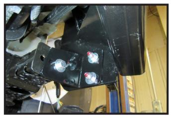
13. Install the 3/8" hardware into the existing holes and fully tighten the bolts. Do this on both sides of the vehicle.
