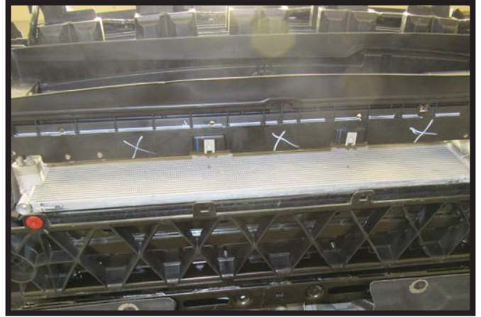
12. Using a reciprocating saw, trim the marked area below the shutters.
