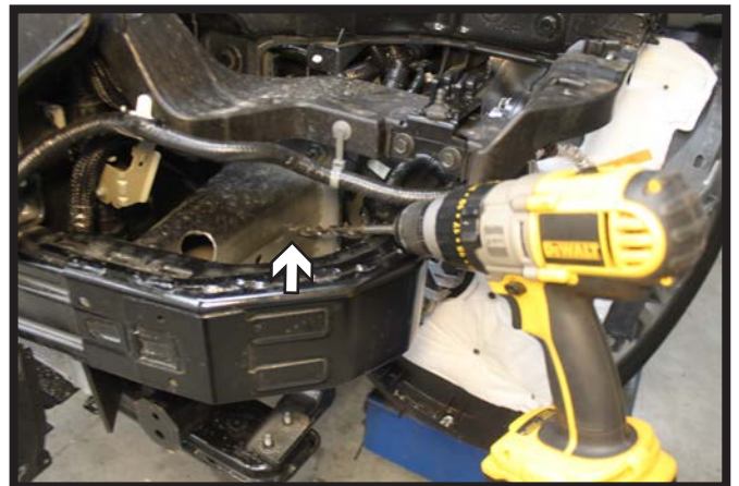
10. Using a 3/8" drill bit, ream out the rear existing hole. Do this on both sides of the vehicle.
