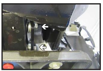
16. Install the 3/8" hardware into the drilled lower support holes, and fully tighten the bolts, using washers as necessary to ensure tightness.
