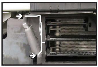
9. Using a reciprocating saw, trim the plastic shielding near the shutters on the passenger side, as shown.
