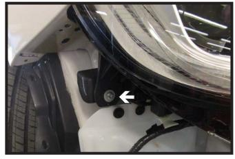
7. Using a T30 Torx, remove the three (3) bolts from the headlight. Do this for both sides of the vehicle.
