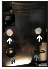
14. Install the lower support plate to the baseplate holes with the supplied 3/8" hardware (white) and fully tighten. Then using a 3/8" drill bit, drill the lower plate holes through the support (gray). Do this on both sides of the vehicle. Fully tighten all hardware.
