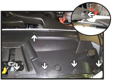
Remove the ten (10) push pins from the fascia cover. There are five (5) on each side. On the driver side, remove one (1) push pin and unhook the cover. Set the cover aside.
