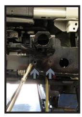
17. Slide the slotted bracket into place and clamp. Install with the supplied 3/8" hardware (white). On the passenger side, using 3/8" drill bit, drill into the bracket (gray). Install with the supplied 3/8" hardware and fully tighten.
