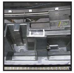
18. **Optional Breakaway:** If installing a breakaway, using a reciprocating saw, cut the marked areas on both the plastic shutter shielding and the fascia. Using a 3/8" drill bit, drill into the baseplate. Install the breakaway with the supplied 3/8" hardware and fully tighten.
