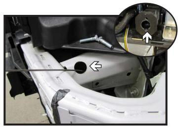
Using a 1-1/4" hole saw, drill access holes in the side of the frame as shown and in the face of the lower support (inset). Do this on both sides of the vehicle.
