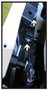
3. Using a 7MM socket, remove the three (3) bolts in front of the tire on the wheel well (white, left). Using a Phillips screwdriver, remove the one (1) screw (gray). Remove the one (1) push pin. Pull the wheel well cover back. Using an 8MM socket, remove the two (2) bolts (white, right). Do this for both sides of the vehicle.
