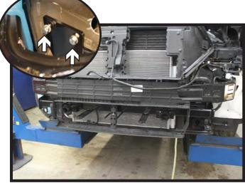
Pull the shielding out away from the vehicle (if applicable) and install the baseplate onto the frame with the 3/8" hardware (inset). Level the baseplate prior to fully tightening the bolts.
