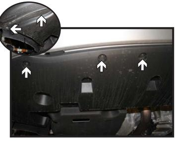
6. Using a 5.5MM socket, remove the ten (10) screws from the underside of the fascia. There are five (5) on each side.
