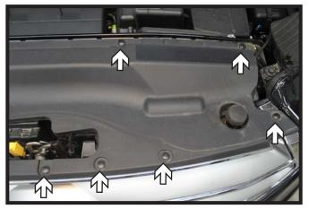
Remove the twelve (12) push pins from the fascia cover. There are six (6) on each side. Set the cover aside.
