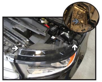
Using a 10MM socket, remove the two (2) screws from the headlight (white). Remove the indicated push pin from the driver side (gray). Disconnect all electrical connections and set the headlight aside. Do this on both sides of the vehicle.
