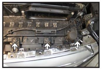
2. Using a 10MM socket, remove the six (6) screws from the top edge of the fascia. There are three (3) on each side.
