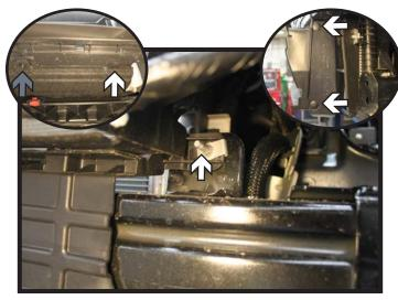
8a. **All Models:** Using a 10MM socket, remove the screw from the shielding just above the bumper.
