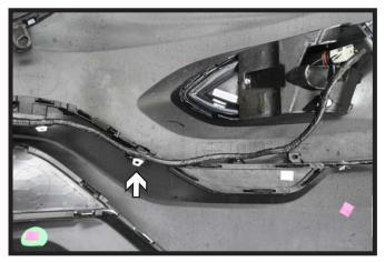
On the backside of the fascia, unhook the loom from the hook. Trim off the hook as necessary for clearance of the baseplate. Do this on both sides of the fascia.
