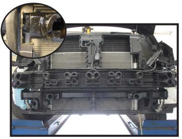
14a.**Non Shutter Models:** Reinstall the shielding, trimming as necessary on the passenger side (inset).
