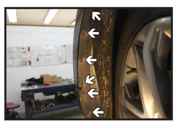
Using a 5.5MM socket, remove the six (6) screws from the edge of the wheel well. Do this on both sides of the vehicle.
