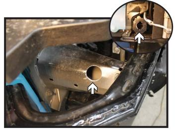
Using a 1-1/4" hole saw, drill access holes in the side of the frame as shown and in the face of the lower support (inset). Do this on both sides of the vehicle.
