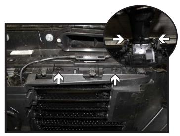
8b. **Shutter Models:** In addition to the 8a steps, using a 10MM socket, remove the four (4) screws from the top of the shielding.
