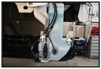
Using a 10MM socket, remove the two (2) screws from the washer reservoir. Disconnect/plug all lines and set the reservoir aside.
