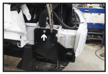
14. Install the baseplate onto the frame, flushing it to the top of the frame. Clamp into place and drill the middle hole thru the frame with a 3/8" drill bit. Install a 3/8" bolt with lock washer into the hole with a 3/8" whiz nut on the inside of the frame lip. Do this on both sides of the vehicle. Level the baseplate and fully tighten the all hardware.
