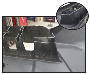
20. On the ends of the lower opening, trim about an inch down along the top side and half way down the side and taper it back to the bottom corner as shown. Do this on both sides of the fascia.
