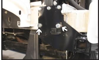
16. Using a 1/2" drill bit, drill the lower two (2) holes thru the frame wall. Install 1/2" bolts with lock washers into the holes with 1/2" nut plates on the inside of the frame. Do this on both sides of the vehicle. Fully tighten all hardware.
