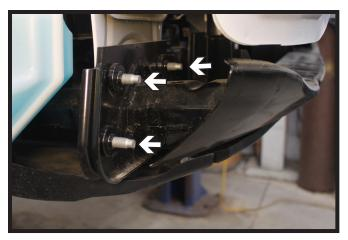
Using a 13MM socket, remove the four (4) bolts from the backside of the crossbar. Do this on both sides of the vehicle. The crossbar will not be reinstalled.
