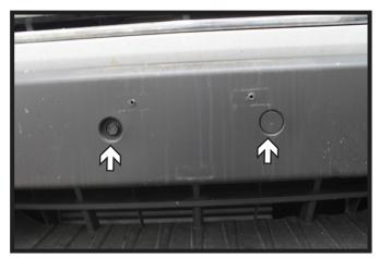
8. Remove the plugs from the fascia. Then using a 13MM socket remove the two (2) screws from the face of the fascia.
