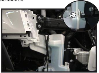
Reinstall the washer reservoir onto the vehicle. Use the supplied 1/4" hardware to attach the reservoir to the bracket as shown.
