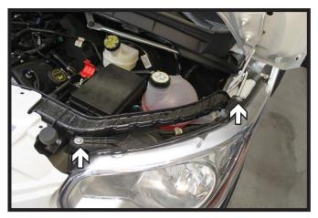
2. Using a T30 Torx, remove the two (2) screws from the headlight. Disconnect any electrical connections and set aside. Do this on both sides of the vehicle.
